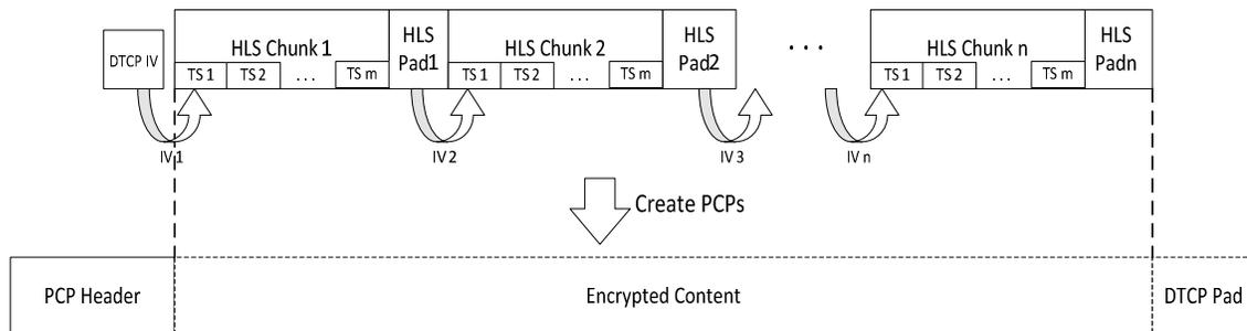
Above picture shows the process of creating PCPs with HLS chunks:
